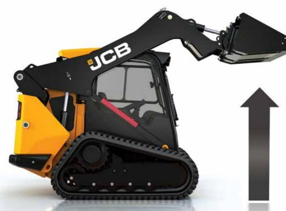
Vertical lift capability provides maximum lift capacity at maximum height and reach, making it the right choice for load and carry operations, including fork work, heavy construction and landscaping.
